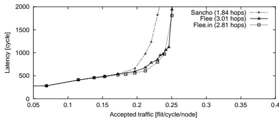
**Figure 21. Incomplete analysis with Viterbi trace on 4x4 mesh under up\*/down\* rule.**
