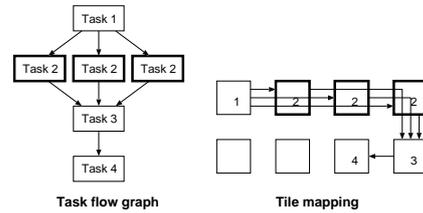
Figure 3. Parallel model. Task 2 is distributed into three nodes and executed in parallel.
