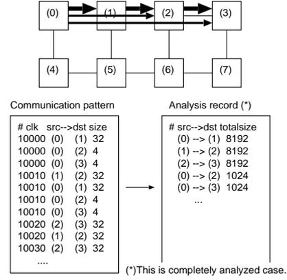
**Figure 4. Communication pattern analysis. Communication pattern of target application is given and all source-destination pairs are sorted in order of total traffic amount.**
