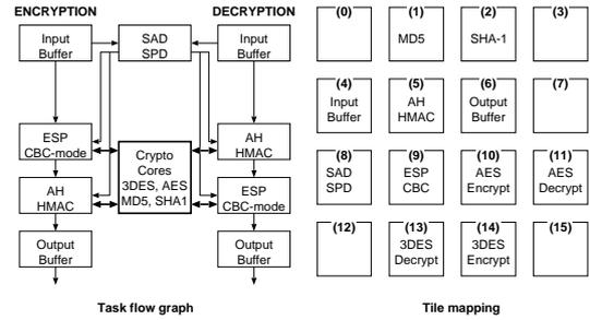
Figure 8. Task flow graph and mapping result for IPsec accelerator.
