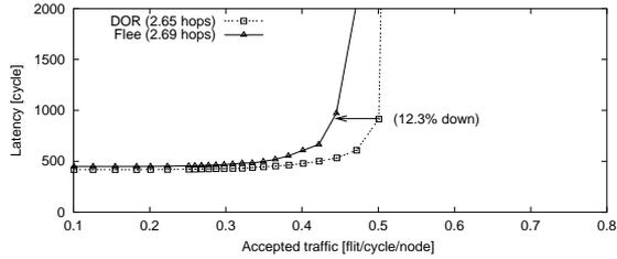
Figure 15. Uniform traffic on 4x4 mesh.
