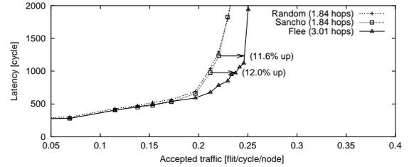
Figure 17. Viterbi trace on 4x4 mesh with no link-fault.
