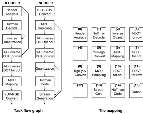
Figure 6. Task flow graph and mapping result for JPEG decoder and encoder.
