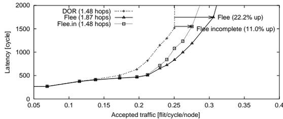
**Figure 20. Incomplete analysis with Viterbi trace on 4x4 torus under Turn-Model.**
