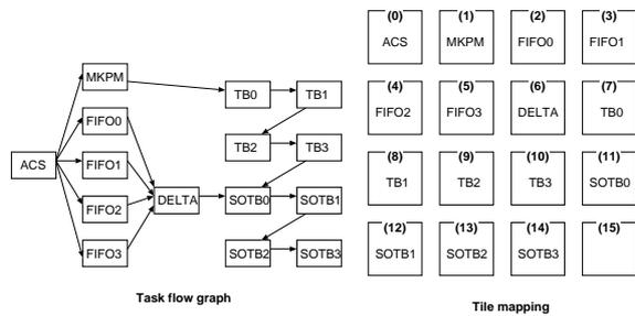
Figure 7. Task flow graph and mapping result for Viterbi decoder.
