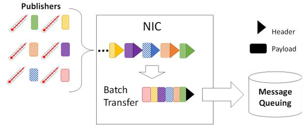
Fig. 2. In-NIC batch processing for incoming messages
