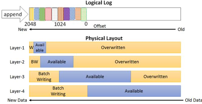
Fig. 4. Logical and physical storage layout in MultiMQC
