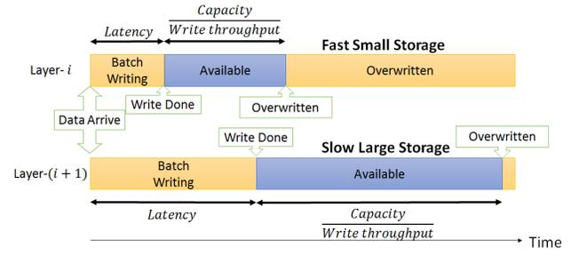
Fig. 5. Example behavior between two layers
