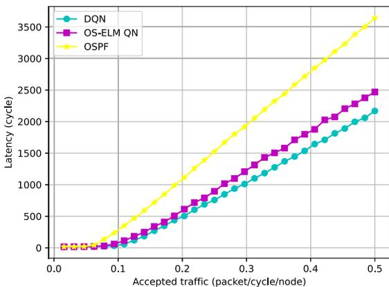
**Fig. 17** Packet transfer latency under bit reverse traffic in 8x8 mesh topology.
