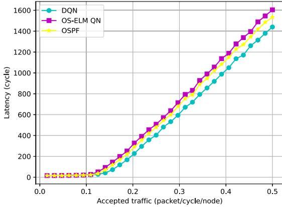
**Fig. 15** Packet transfer latency under uniform traffic in 8x8 mesh topology.
