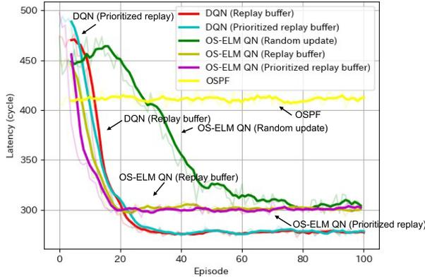
**Fig. 9** Packet latency vs. training episodes of different methods. Y-axis shows the total number of cycles to transfer a packet.
