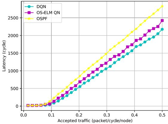
**Fig. 16** Packet transfer latency under transpose traffic in 8x8 mesh topology.
