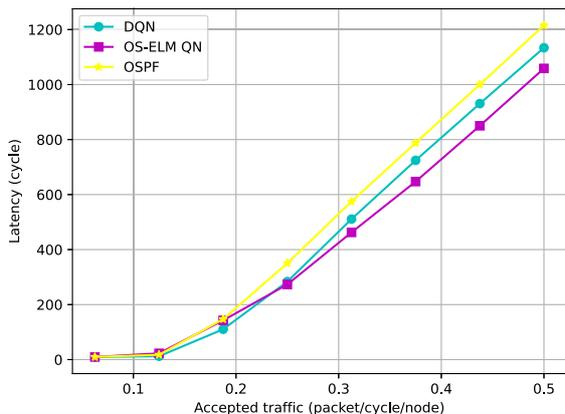
**Fig. 11** Packet transfer latency under transpose traffic in 4x4 mesh topology.
