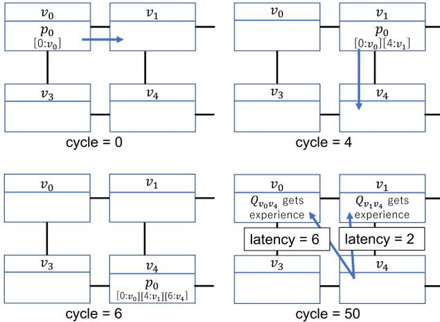
Fig. 5 Routing example.  $p_0[x:v_i]$  means  $p_0$  reached  $v_i$  at  $x$  cycle.
