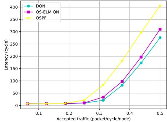
**Fig. 10** Packet transfer latency under uniform traffic in 4x4 mesh topology.
