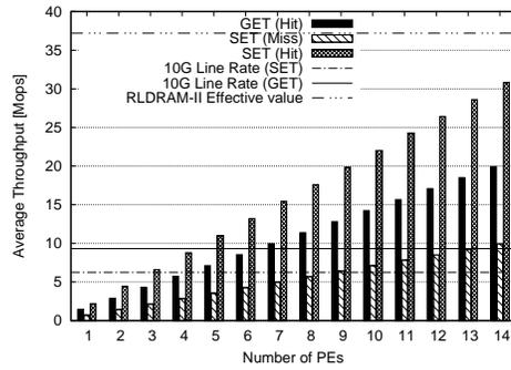
Fig. 6. Aggregated throughput with multiple string PEs on NetFPGA-10G.
