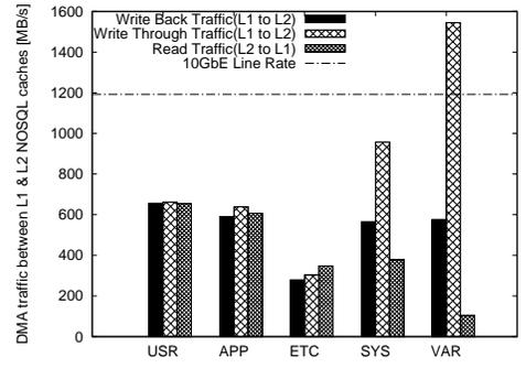
Fig. 7. DMA traffic between L1 and L2 NOSQL caches (write-back vs. write-through).
