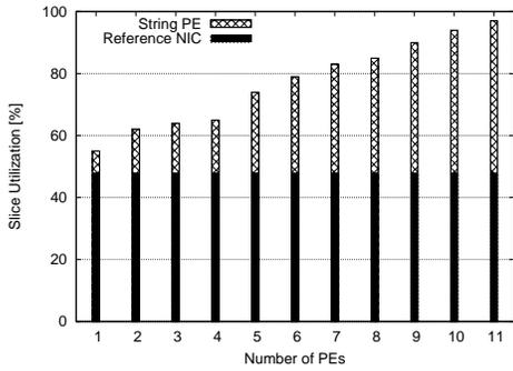
Fig. 5. Area utilization on Virtex-5 XC5VTX240T.
