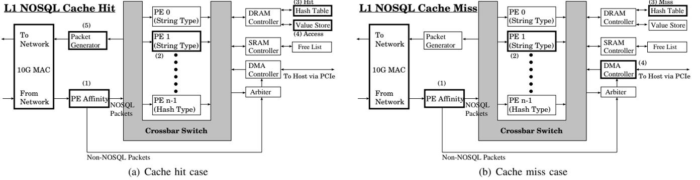
Fig. 2. Heterogeneous multi-PE design of L1 NOSQL cache and its behavior (two cases).
