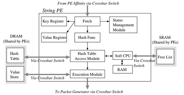
Fig. 4. KVS PE core architecture.
