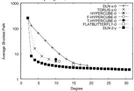
Figure 3. Average shortest path length vs. degree for non-random topologies and for random shortcut DLN topologies ( $N=2^{10}$  vertices).
