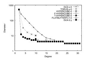
Figure 2. Diameter vs. degree for non-random topologies and for random shortcut DLN topologies ( $N=2^{10}$  vertices).
