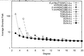
Figure 11. Average shortest path length vs. degree for random shortcut topologies generated using different base topologies ( $N=2^{10}$  vertices).
