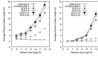
Figure 27. Average cable length vs. N for non-random topologies and random shortcut DLN with distributed switch layout.
