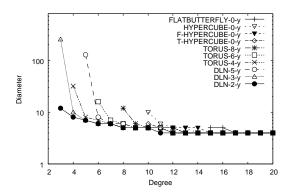
Figure 10. Diameter vs. degree for random shortcut topologies generated using different base topologies ( $N=2^{10}$  vertices).
