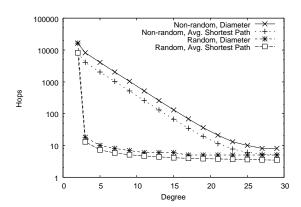
Figure 1. Diameter and average shortest path length vs. degree for a  $2^{15}$ -vertex ring topology with non-random shortcuts and a ring topology with random shortcuts.
